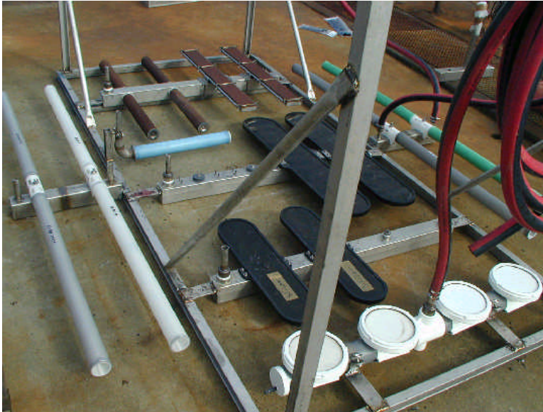
Picture 1: test rack with diffusers of OTT (long tubes), and other European diffuser technologies including rectangular plates, short tubes, discs and oval plates
